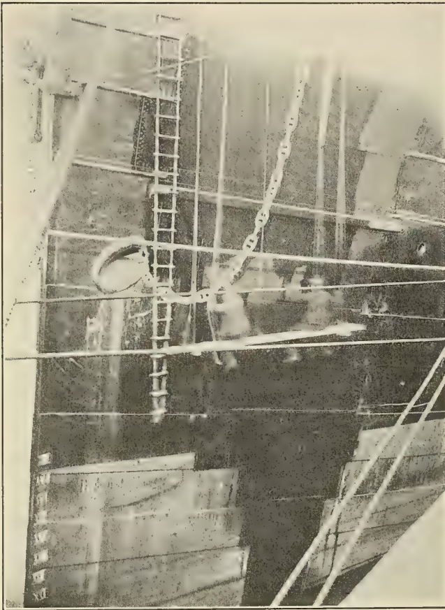
THE MONGOLIAN PATCHED UP AFTER THE COLLISION.
